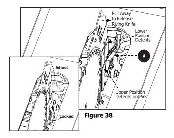
**AWARNING: DO NOT** operate saw unless riving knife is securely clamped in the raised position for through cutting or the lowered position for non-through cutting.
